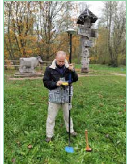
Fig. 5. Detailed field works for the arrangement of GCP points in Mantagailiškis and Karajimiškis villages.
